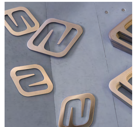
__ parts as small as 50x50mm can be easily rounded on this machine
