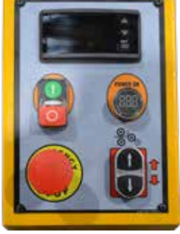
Opsiyonel dijital kumanda paneli Optional control panel with digital readout
