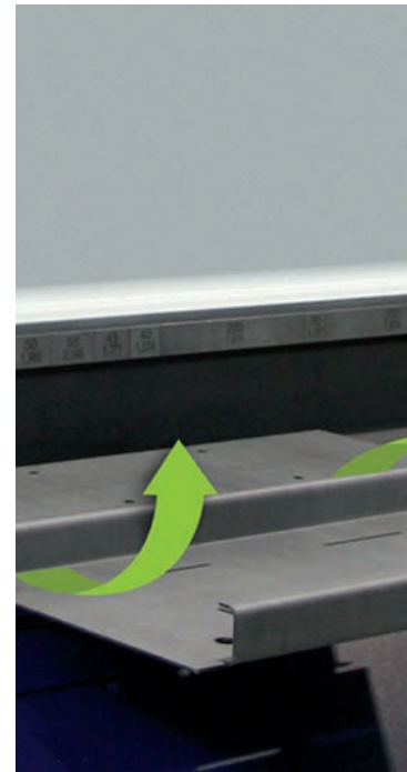
Up-and-Down function: counter folds without turning the sheet
