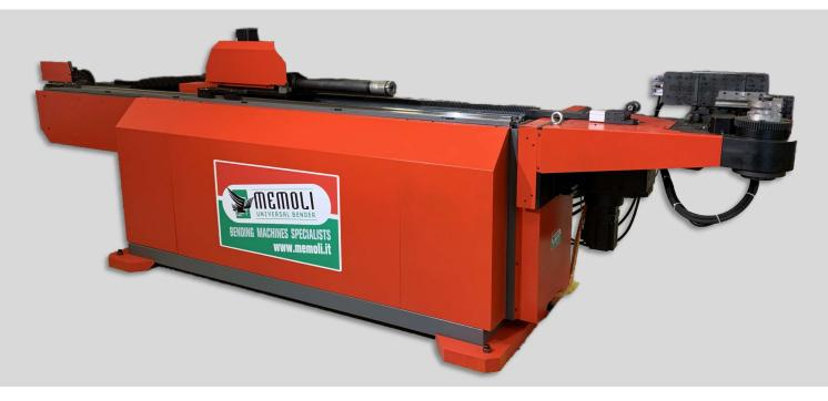
The ACH range is the series of **3-axis CNC bending machines** for the linear bending of tubes up to 65 mm diameter. The bending machines of the ACH series are fully automatic bending machines with CNC 3 axes: **bending** (Y axis), **advancement** (X axis) and **rotation** (Z axis).
