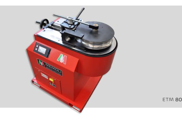
The ETM series is equipped with state of the art technologies meant to bend with or without mandrel tubes and profiles, and capable of bending both in right and left direction. It allows to bend tubes with a range diameter **from 8 mm up to 168 mm** and it can make curves **over 180°** with top finish quality for a minimum bending radius of 3 x the tube diameter. Every ETM machine is manufactured from single welded steel block and the toolings are machined from solid steel.
