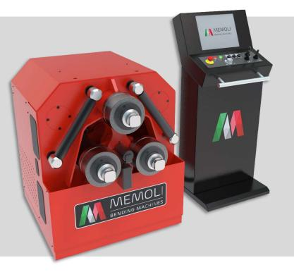
The MEK 60-R **three-roll hybrid profile bender** was designed to meet the demands of an increasingly demanding Customers base, with the need to bend all types of profiles and tubes with **accuracy** and very tight tolerances. The three driving rolls are driven by a powerful electric gearmotor that guarantees high positioning accuracy, while the independent planetary movement of the two bottom rolls is provided by two powerful hydraulic cylinders.
