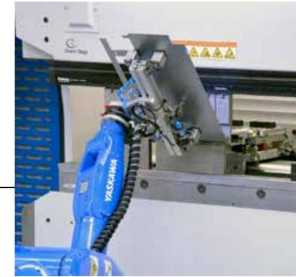
**PR-CELL**, is the independent solution for automated bending process, from feeding, handling and palletizing. Various control systems, security and automatic tools changes are possible.
