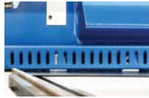
Rubber pads under hold down to avoid any markings or scratching of sheets
