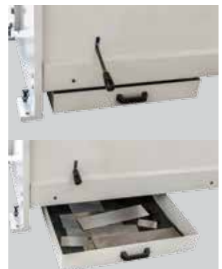
Front-side collection box to collect small parts to the front: parts up to 300mm drop into the wheel tray located in the front of the machine
