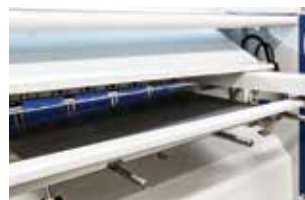
Extended holding arms keep the sheet always at the same level over the entire length
