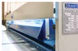
Bright LED cutting line illumination
