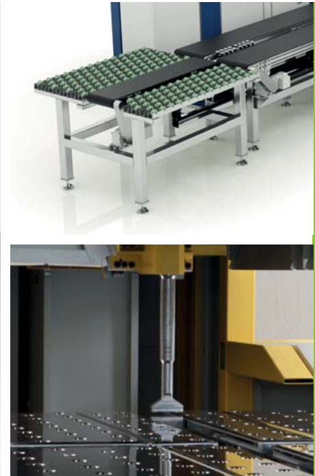
Customized solutions Above: Roller table for unloading the final product Below: Gripper arm of manipulator positions the sheet precisely, controlled via high-precision camera systems. .
