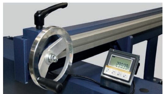
Optional: Manual back gauge, adjustable from the front, with digital readout (standard equipment)
