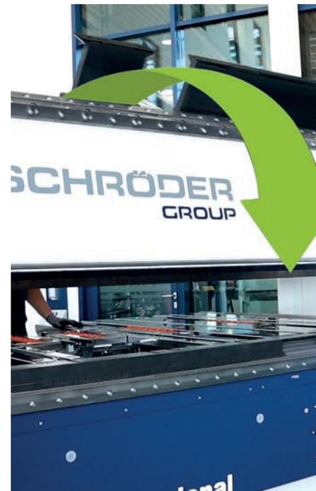
The rotating clamping beam offers a second set of tools and an alternative machine geometry. (New: Clamping beam directly driven with servo motors)
