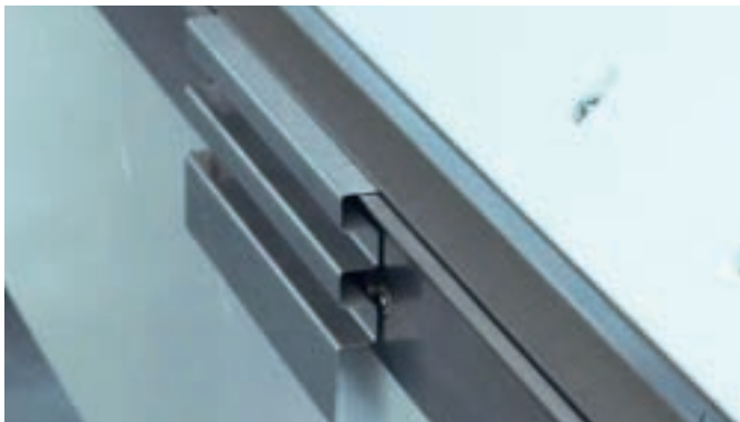
Thanks to the set back folding beam with a cranked folding blade trapezoidal sheets and profiles with standing seams are very easy to bend.
