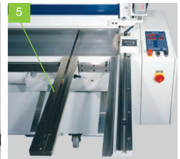
Movable sheet support with T-slots on linear guide
