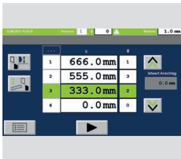
NC positioning gauge Classic Cut with 9-step program.
