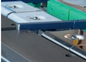
Bottom beam blade with finger grooves
