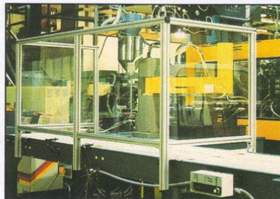
Guard Mounted to Conveyor System and Machine
