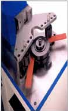
■ Flat plate edge bending tool for up to 2"x1/2"
